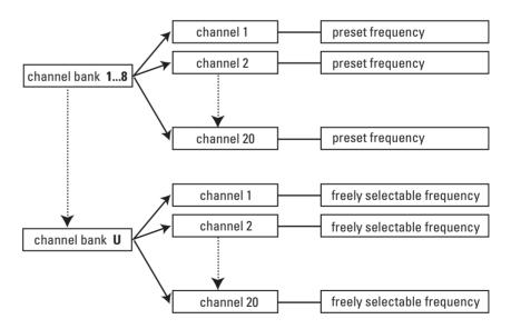
Each of the channels in the channel banks "1" to "8" has been factory-preset to a receiving frequency (see enclosed frequency table). These receiving frequencies cannot be changed but have been preset so that e.g. country-specific regulations on frequency usage are taken into account.
